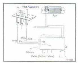
Fig 8. Comfort control wiring diagram
